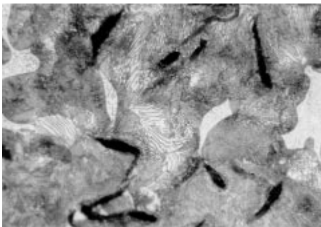
Fig. 11 Microstructure of alloy D near chill end (cast with subzero end chill). 500×
