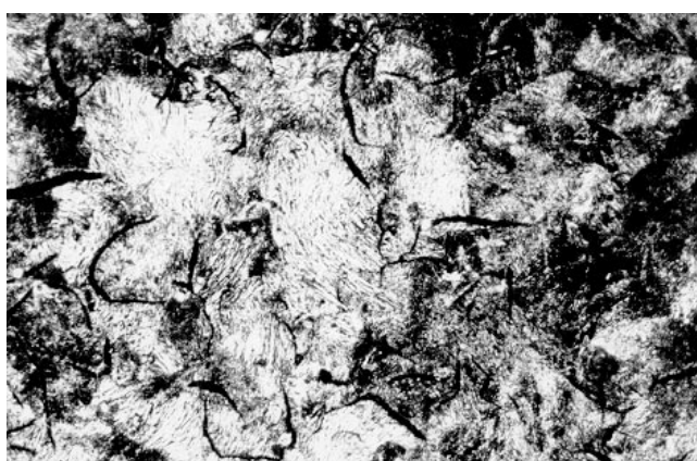
Fig. 10 Microstructure of alloy C near chill end (cast with water-cool end chill). 500×
